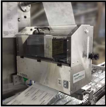
MLP on a HFFS medical device packaging line
