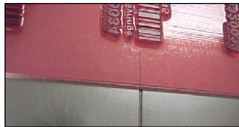
Figure 7-Correct Vertical Plate Alignment
