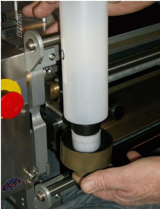
Figure 16-Inserting the Ink Cartridge
