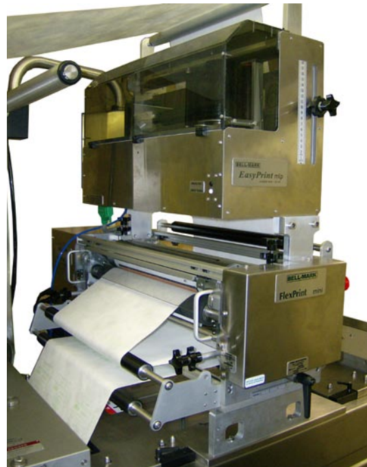
Figure 2-Mounted Flexprint and EasyPrint MLP Combination
