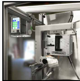
Mounted on a Continuous flow wrapper
