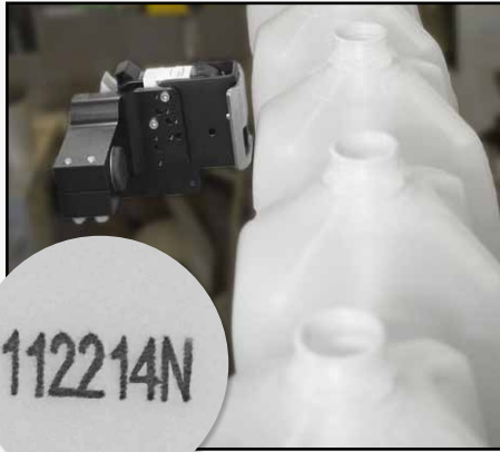
Conveyor Mount Printing on Plastic Bottles
