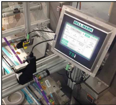
Mounted to a Continuous Motion Flow Wrapper
