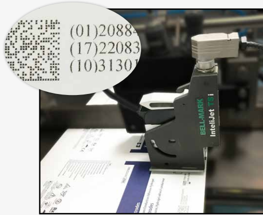
Mounted to Horizontal Pouch Seal Machine
